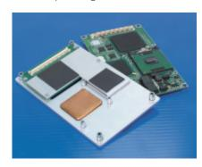
Gap Pad 1500 has an ideal filler blend that gives its low-modulus characteristic that maintains optimal thermal performance yet still allows for easy handling. The natural tack on both sides of the material allows for good compliance to adjacent surfaces of components, minimizing interfacial resistance.
